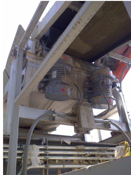
FIELD IMAGE: Vibratory Feeder in use at a Plastics Recycling Plant, powered by two (RE) Rotary Electric Motors
