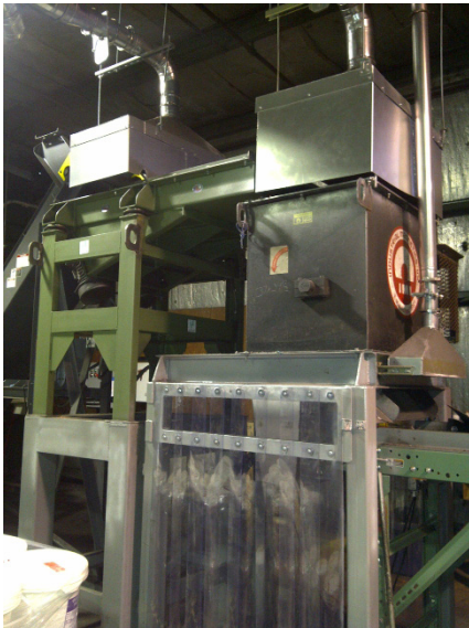
FIELD IMAGE: Vibratory Feeder in use at a Battery Recycling Plant, to consistently feed materials through processing
